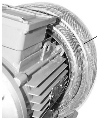
Fig. 5.10: Cleaning the compressed air/oil cooling unit
