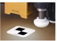
ARGHON recognizes details size less than **0.1 mm**. It enables a better recognition of ROT (Reference Optical Tag) for automatic hide re-centering.
