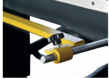
Kolay ayarlanabilen arka dayama Back gauge with easy setting
